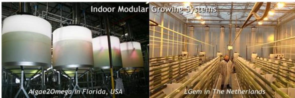
LGem is growing nannochloropsis for omega3 oils in Den Haag, the Netherlands. Inside large high-tech warm greenhouses, widely used for growing crops, sunlight illuminates the algae cultures during sunny days and can be supplemented with artificial lighting during cloudy days and in the off season with shorter days. (LGem, 2012)
